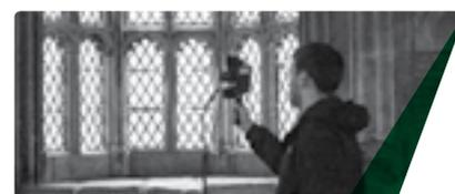
**Rapid scanning time** – within minutes anyone can be operating the ZEB-REVO, and our intelligent software (which uses the most established and robust SLAM mapping algorithm in the industry) can map a 3-storey building in just 30 minutes to an accuracy level of  $\pm 15\text{mm}$ , or map a 10,000 m<sup>2</sup> (105,000 sq. ft.) depot in under an hour. Walk through your target survey environment to record more than 43,000 measurement pts/sec, and from scan to full 3D BIM model in under an hour!
